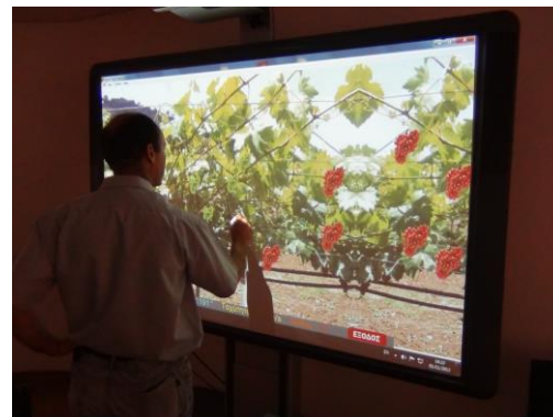
Figure 2c. Selecting targets (grape clusters) using a digital pen on a smart interactive whiteboard
