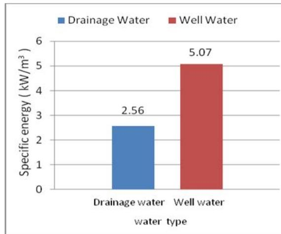
Fig.(5) the effect of feed water type, feed flow rate on the Specific energy.
