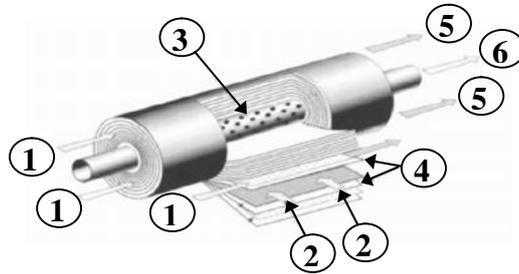
(1) Feed Water (2) Permeate Flow toward Collection Tube (3) Perforated Collection Tube. (4) Membrane. (5) Concentrated water ( Brine ) . (6).Desalinated water (Permeate ) .
