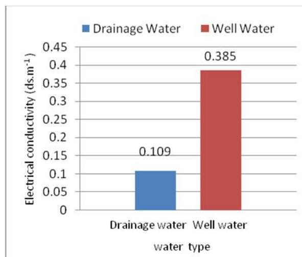
Fig.( 6 ) The Effect Of Water type and Feed Flow Rate On The Electrical Conductivity Of Desalinated Water.
