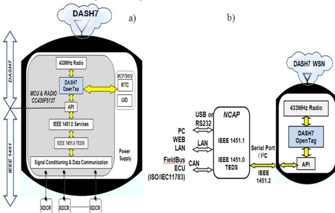
Figure 2. a) DASH7-based WSN node with IEEE 1451 STIM functionality, and b) DASH7-based WSN node interface with a IEEE 1451 NCAP.
