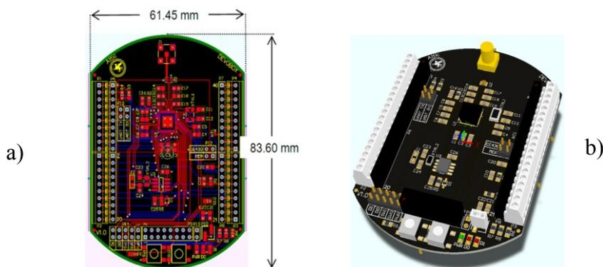
Figure 1. The printed circuit board (a) and a 3D view (b) of the DASH7 node
