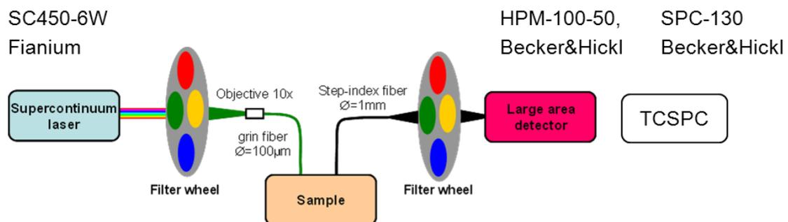
Figure 2. Scheme of the system set-up for TRS. TCSPC: time-correlated single photon counting.
