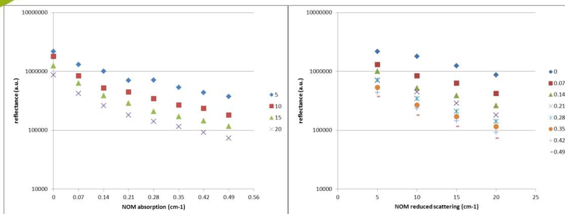
Figure 4. Diffuse reflectance readings from the multipath CW sensor as a function of the absorption coefficient for different values of the scattering coefficient (left) and as a function of the reduced scattering coefficient for different values of the absorption coefficient (right).
