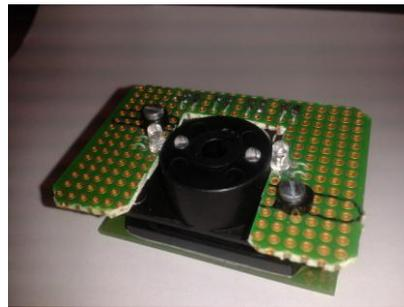
Figure 1. Photo of head of the multi-path CW sensor.
