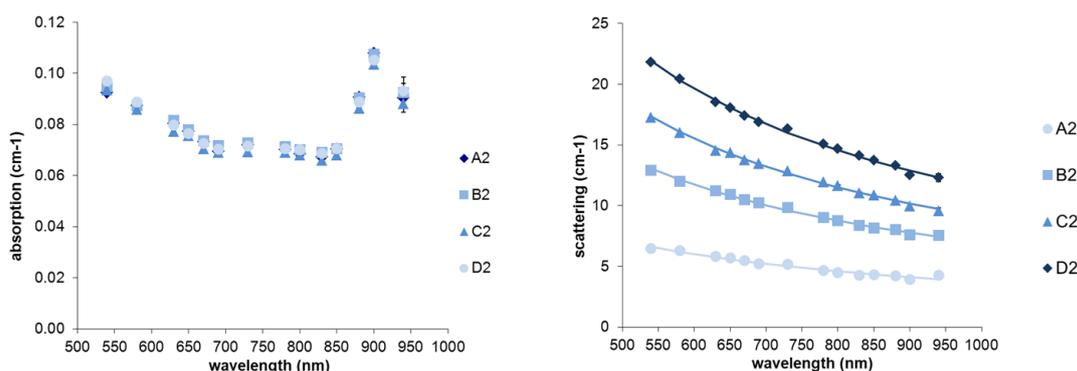
Figure 3. Absorption (left) and reduced scattering (right) spectra of phantoms A2, B2, C2 and D2. The continuous line is the best fit of the reduced scattering spectrum with the Mie approximation (Mourant et al., 1997).
