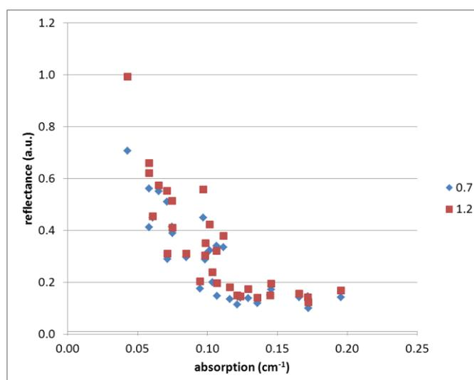
Figure 5. Diffuse reflectance readings with the CW sensor taken on apples at 0.7 and 1.2 cm as a function of the absorption coefficient as measured by TRS.
