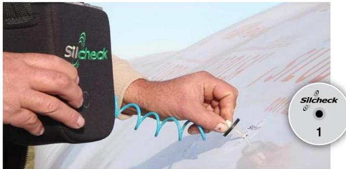
Figure 2. Meter monitoring the CO<sub>2</sub> concentration of a silobag, with the detail of the rubber patch used for inserting the needle.
