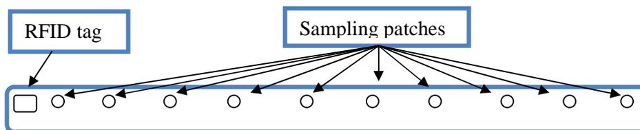
Figure 1. Schematics of the allocation of the RFid tag and the sampling patches in a standard silobag.
