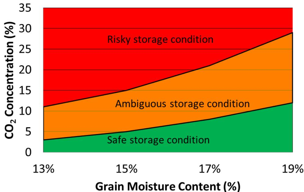
Figure 3. Chart showing the regions considered as risky, ambiguous and safe based on the grain moisture content and the CO<sub>2</sub> measurement for a generic grain.
