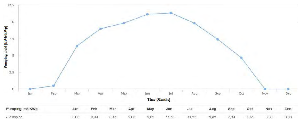
Figure 10 Monthly pumping yield of the PV pumping system (Alexandria Romania)
