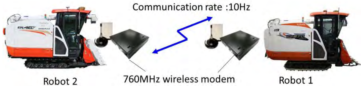
Figure 3. A communication system between combine robots by wireless modems.
