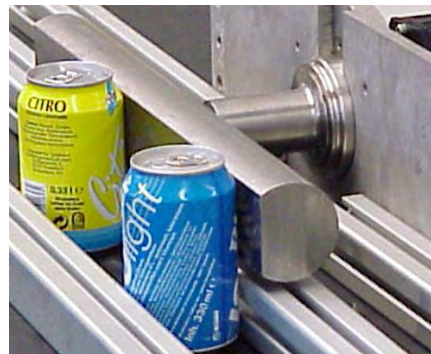
Figure 1. Detection of beverage Cans for Leak by ultrasound
