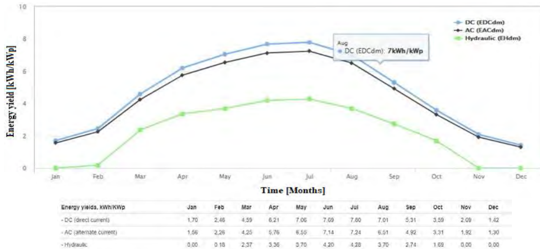
Figure 9 Monthly energy yield of the PV pumping system irrigation (Alexandria, Romania)
